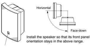
Install with the logo mark located at the bottom of the front panel.
